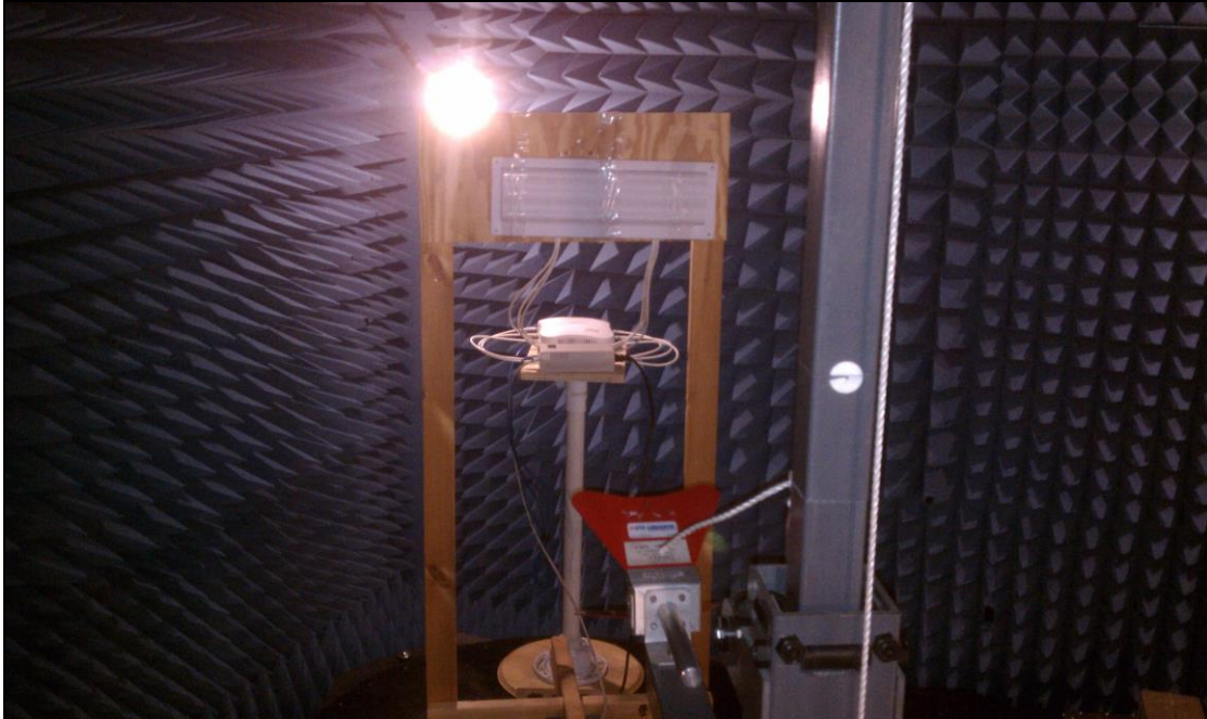
Photograph 7. Radiated Spurious Emissions, Test Setup, HF Patch Antenna
