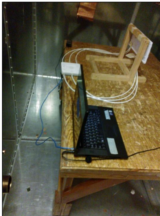
Photograph 3. Conducted Emissions, 15.207(a), Test Setup, Rear View
