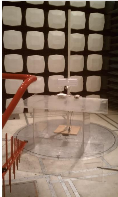
Photograph 6. Radiated Spurious Emissions, Test Setup, LF Patch Antenna
