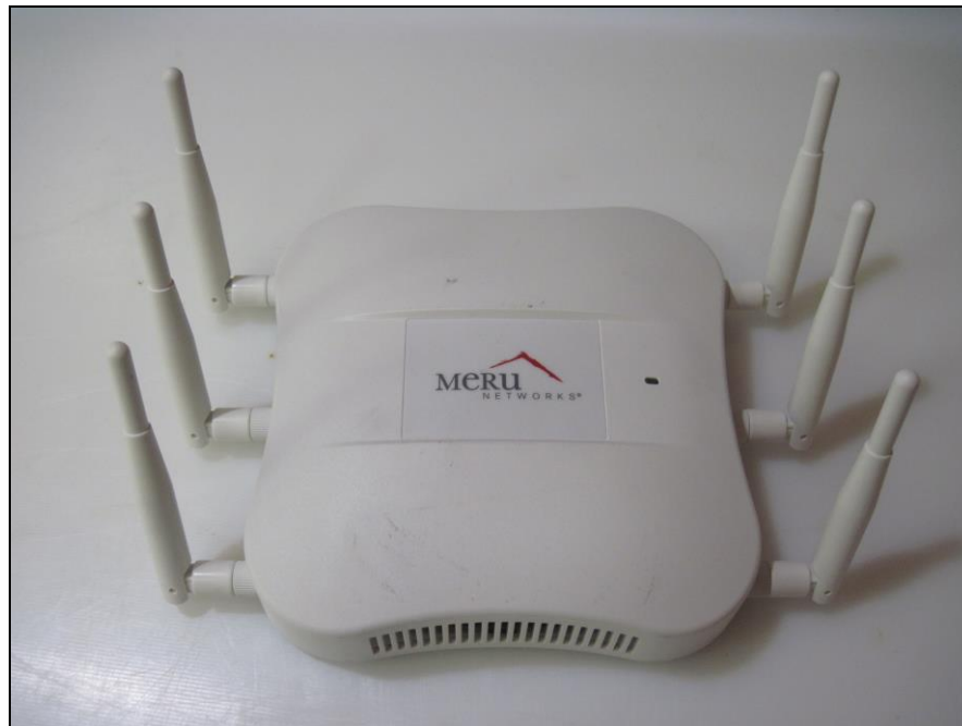
Photograph 1. Meru Networks, Inc. Dual Radio 802.11abgn 3x3 Access Point with External Antenna - AP332e
