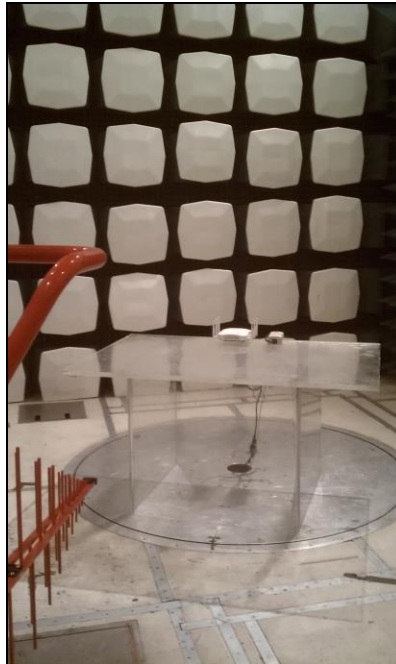
Photograph 4. Radiated Spurious Emissions, Test Setup, LF Dipole Antenna
