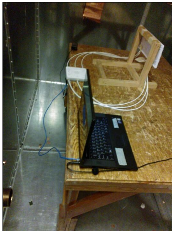
Photograph 2. Conducted Emissions, 15.207(a), Test Setup, Rear View
