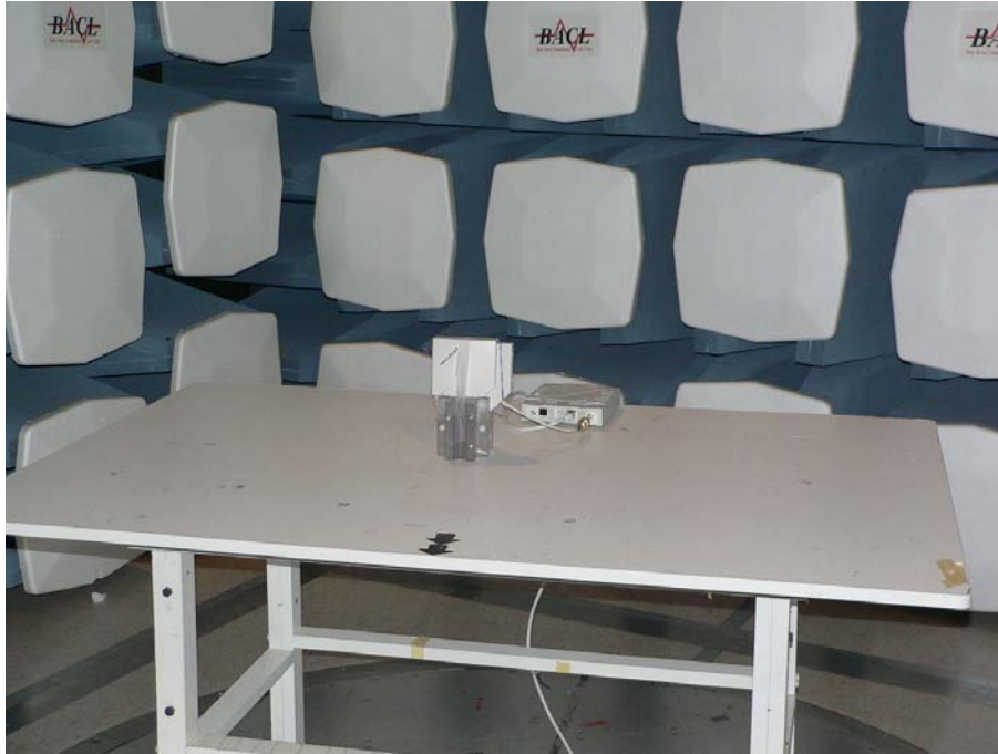
Radiated Spurious Emissions – Front View
