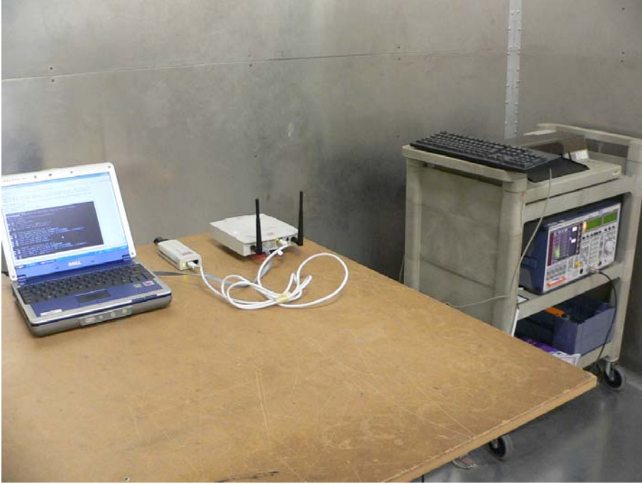
Conducted Emission – Rear View
