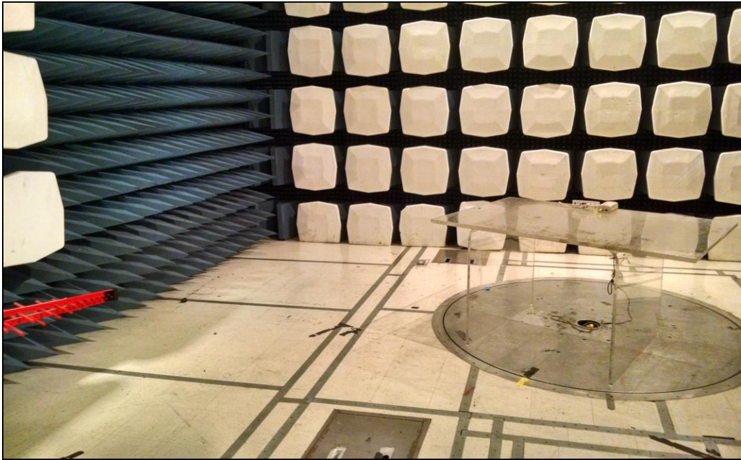
Photograph 5. . Radiated Spurious Emissions, Test Setup, 30 MHz – 1 GHz
