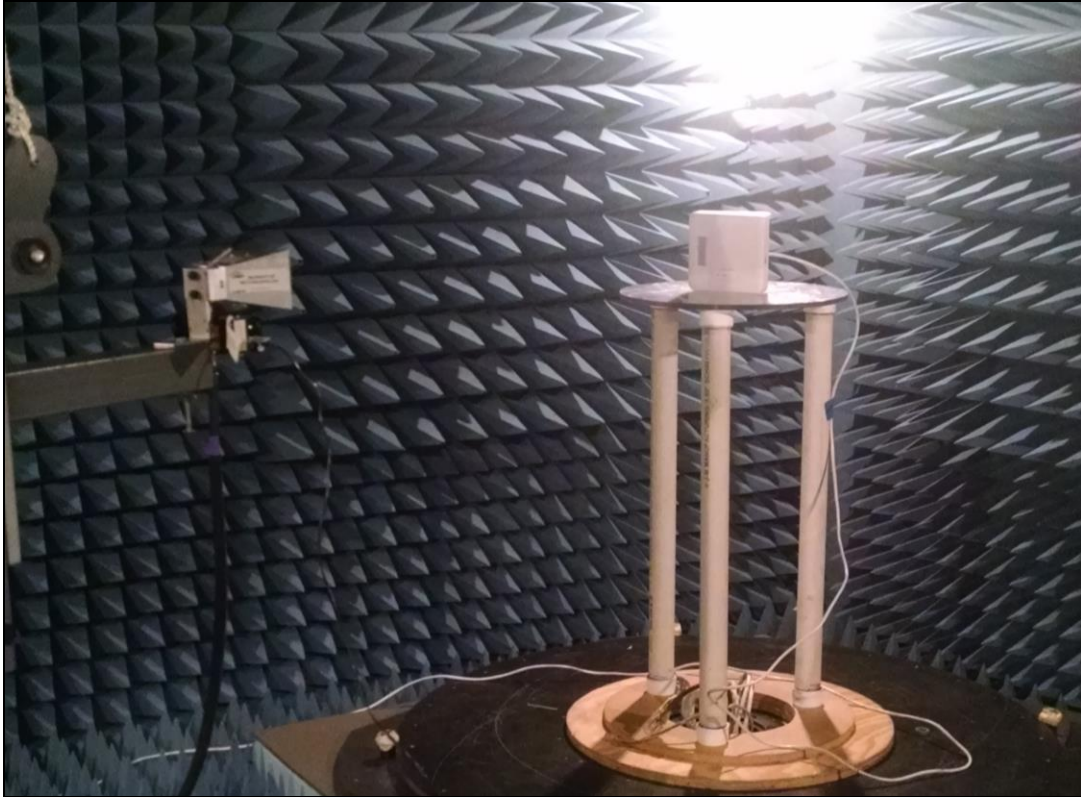
Photograph 7. Radiated Spurious Emissions, Test Setup, 18 MHz – 40 GHz
