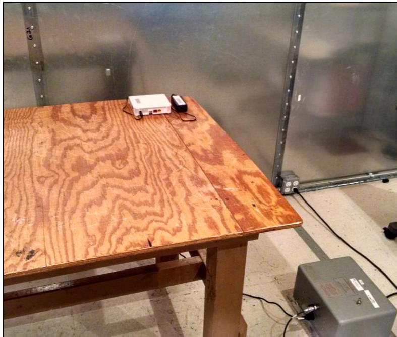
Photograph 3. Conducted Emissions, Test Setup, AC/DC
