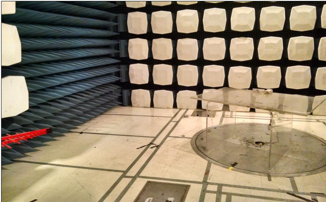
Photograph 4. Radiated Spurious Emissions, Test Setup, 30 MHz – 1 GHz
