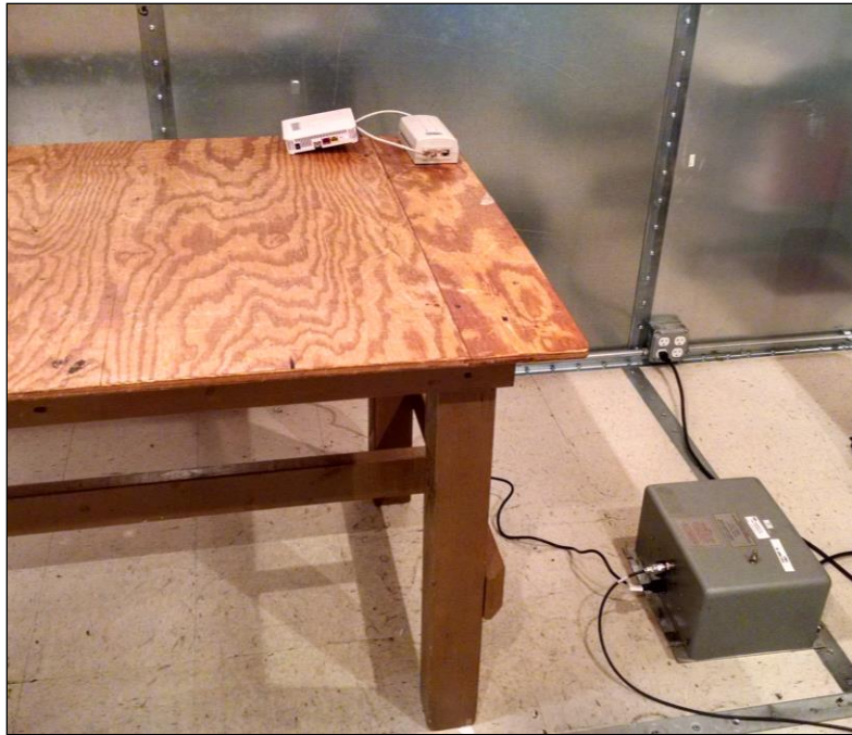
Photograph 1. Conducted Emissions, Test Setup, PoE
