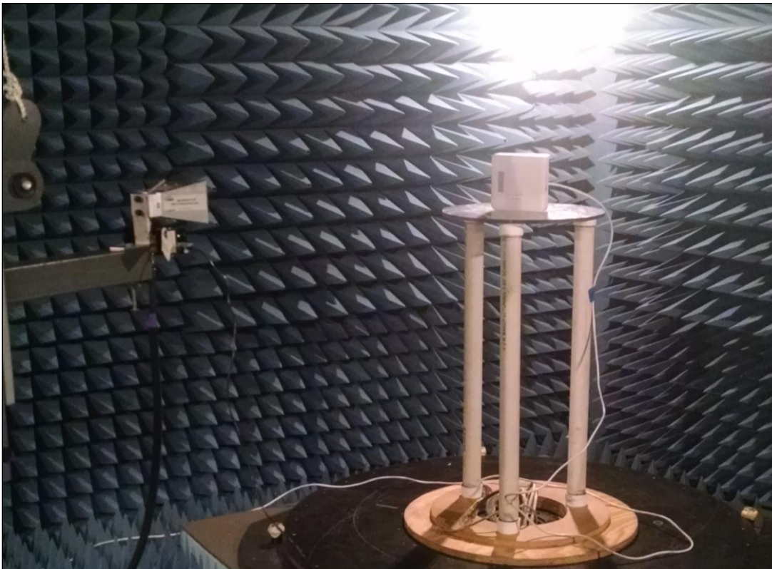
Photograph 6. Radiated Spurious Emissions, Test Setup, 18-40 GHz
