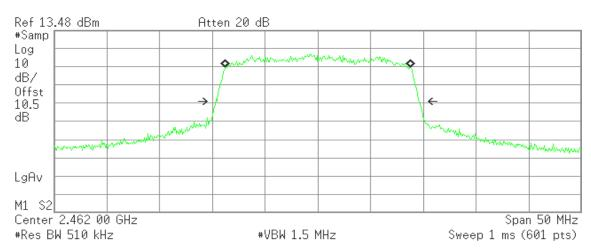
Occupied Bandwidth 17.4806 MHz Occ BW % Pwr 99.00 % x dB -26.00 dB
