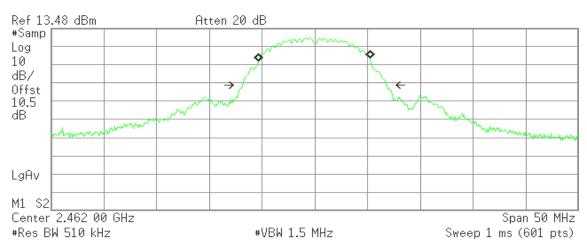
Occupied Bandwidth 10.5342 MHz Occ BW % Pwr 99.00 % x dB -26.00 dB
