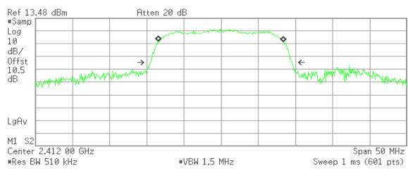
Occupied Bandwidth 16.7444 MHz Occ BW % Pwr 99.00 % x dB -26.00 dB
