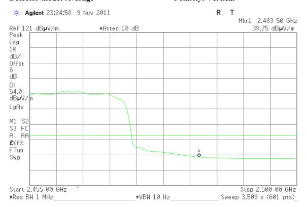
Detector mode: Peak Polarity: Horizontal
