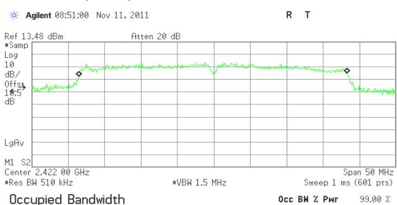
Transmit Freq Error -146.977 kHz x dB Bandwidth 50.000 MHz\*
