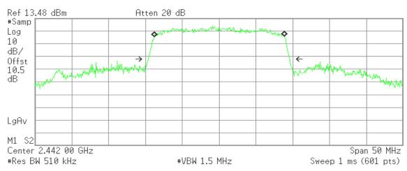
Occupied Bandwidth 17.5453 MHz Occ BW % Pwr 99.00 % x dB -26.00 dB
