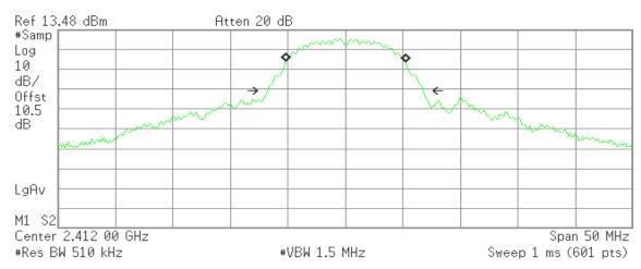
Occupied Bandwidth 10.4443 MHz Occ BW % Pwr 99.00 % x dB -26.00 dB
