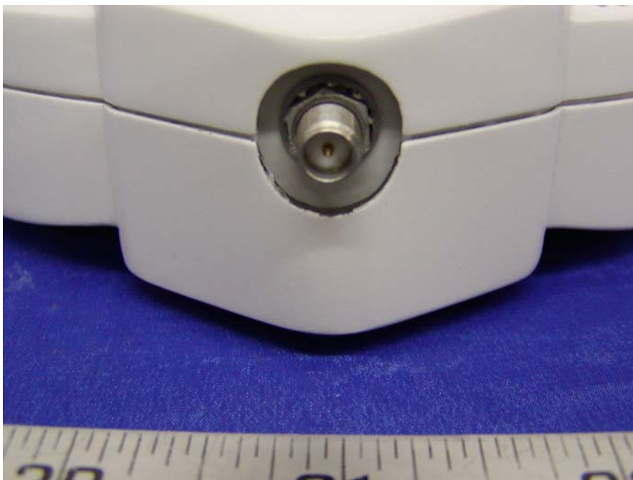
Antenna Connector View, EUT Side (Reverse SMA)
