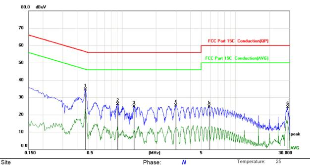
Limit: FCC Part 15C Conduction(QP) Power: AC 120V/60Hz Humidity: 55 %
