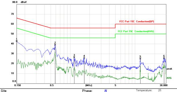
Limit: FCC Part 15C Conduction(QP)
