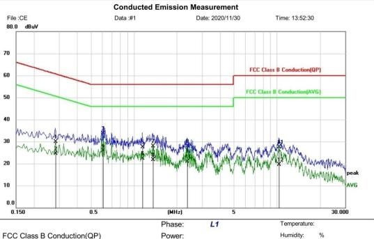
Limit: FCC Class B Conduction(QP) EUT: TWS Bluetooth earphones
