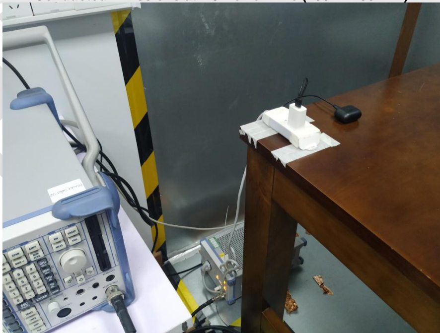
Conducted Emissions at AC Power Line (150kHz-30MHz)
