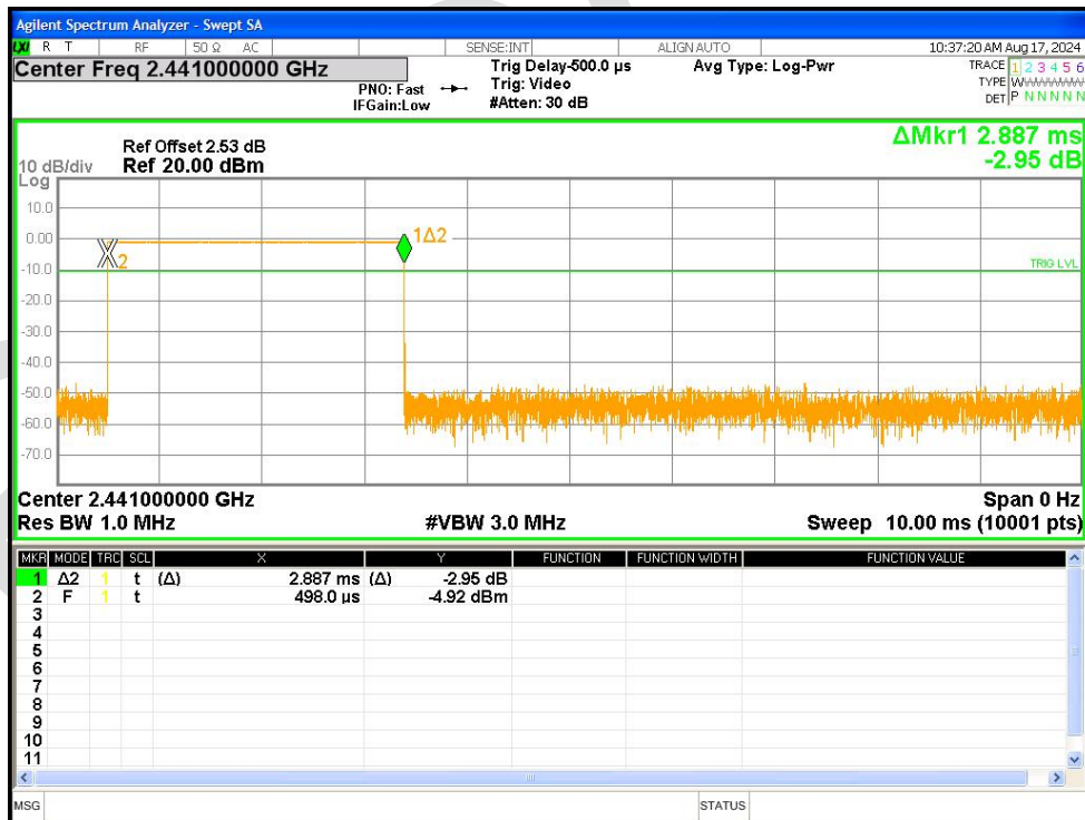
Dwell NVNT 1-DH5 2441MHz Ant1 Accumulated
