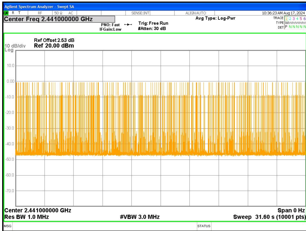
Dwell NVNT 1-DH5 2441MHz Ant1 One Burst
