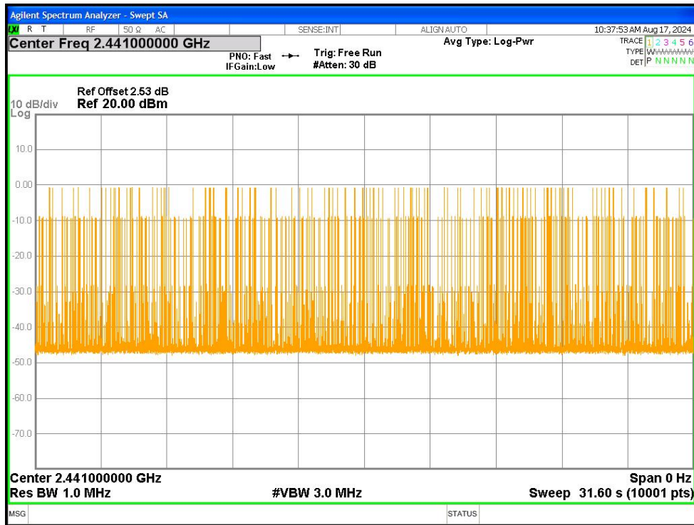
Dwell NVNT 2-DH5 2441MHz Ant1 One Burst
