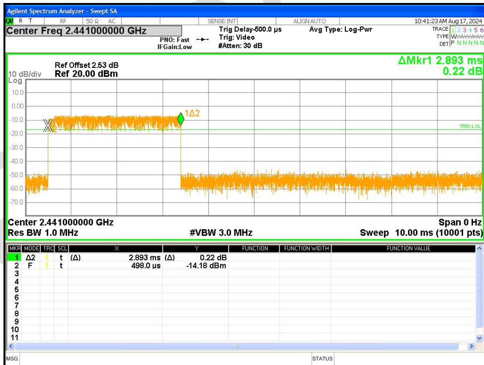
Dwell NVNT 3-DH5 2441MHz Ant1 Accumulated
