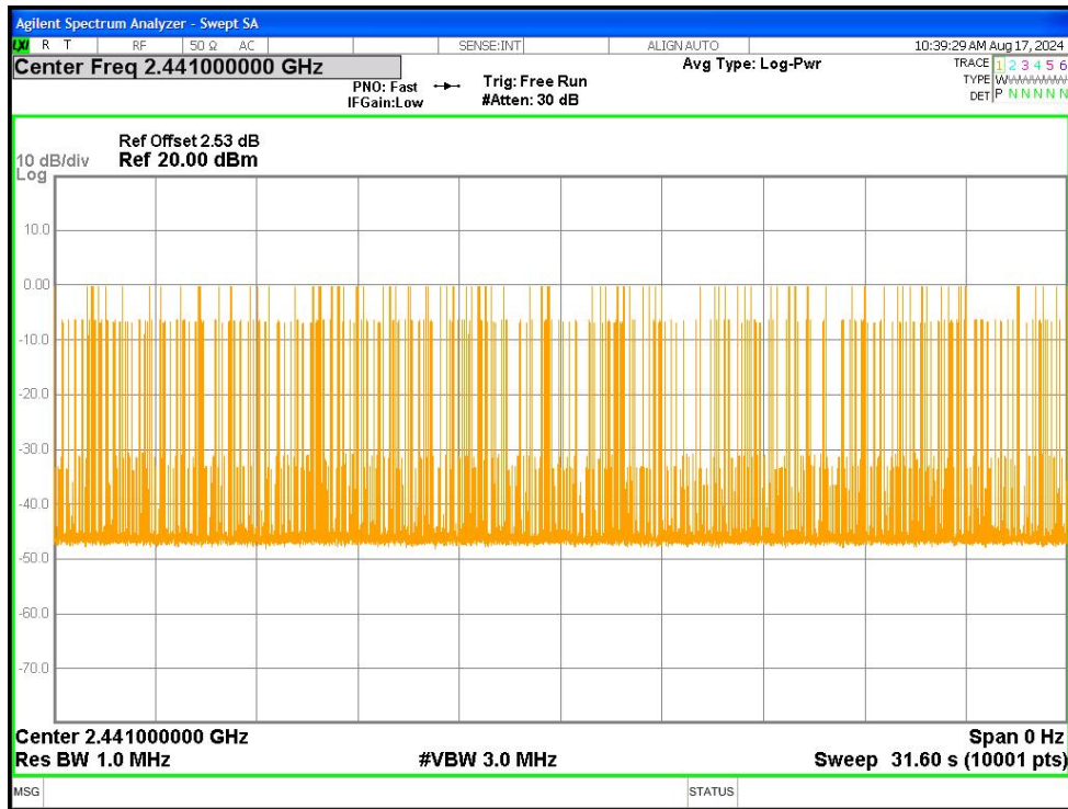
Dwell NVNT 3-DH5 2441MHz Ant1 One Burst
