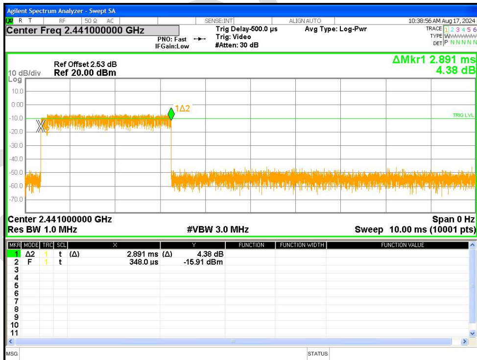
Dwell NVNT 2-DH5 2441MHz Ant1 Accumulated
