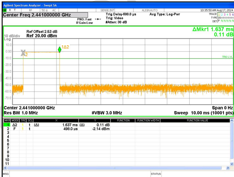
Dwell NVNT 1-DH3 2441MHz Ant1 Accumulated
