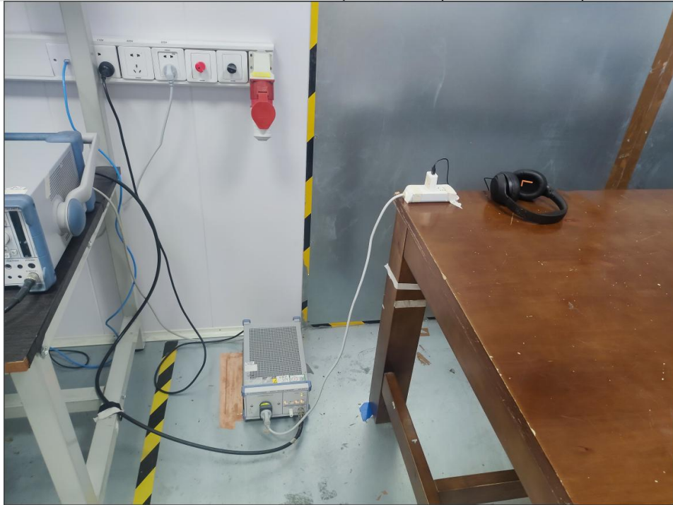
Conducted emissions at AC power line (150kHz-30MHz)
