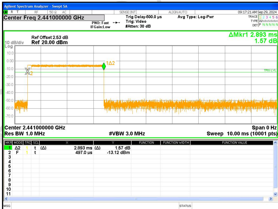
Dwell NVNT 2-DH5 2441MHz Ant1 Accumulated
