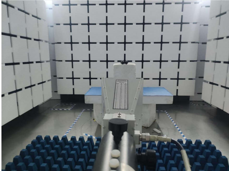
Radiated Emissions (above 1GHz)
