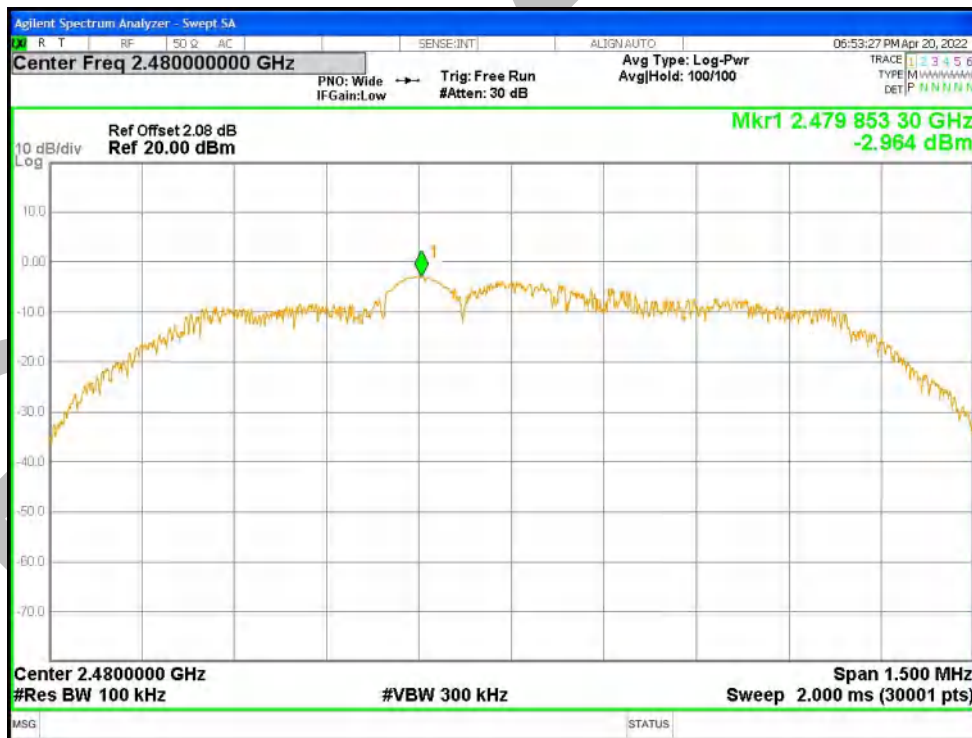
Tx. Spurious NVNT 2-DH1 2480MHz Ant1 Emission
