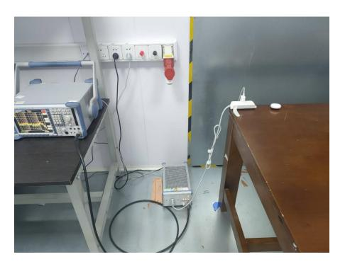
Conducted Emissions at AC Power Line (150kHz-30MHz)
