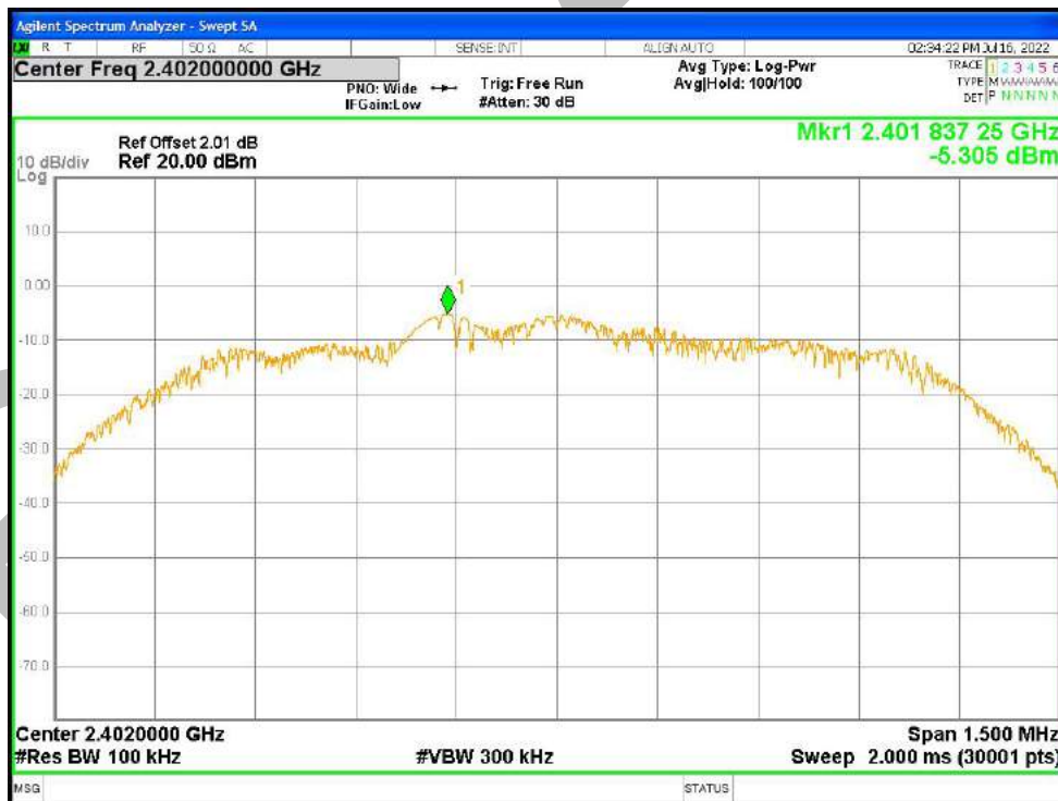
Tx. Spurious NVNT 2-DH1 2402MHz Ant1 Emission
