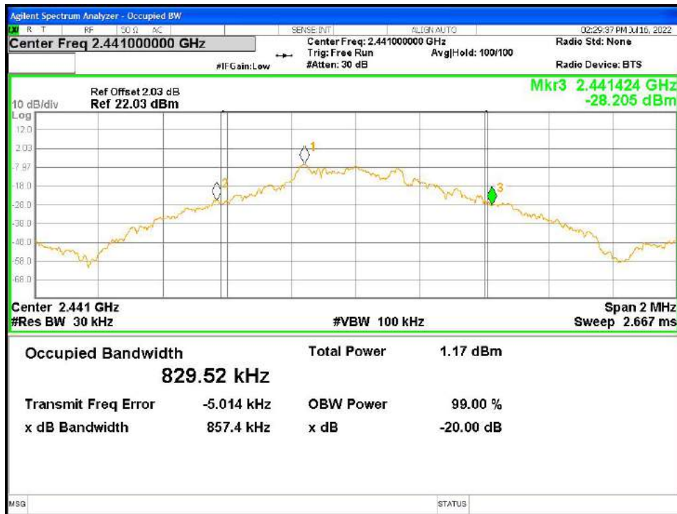
-20dB Bandwidth NVNT 1-DH1 2480MHz Ant1
