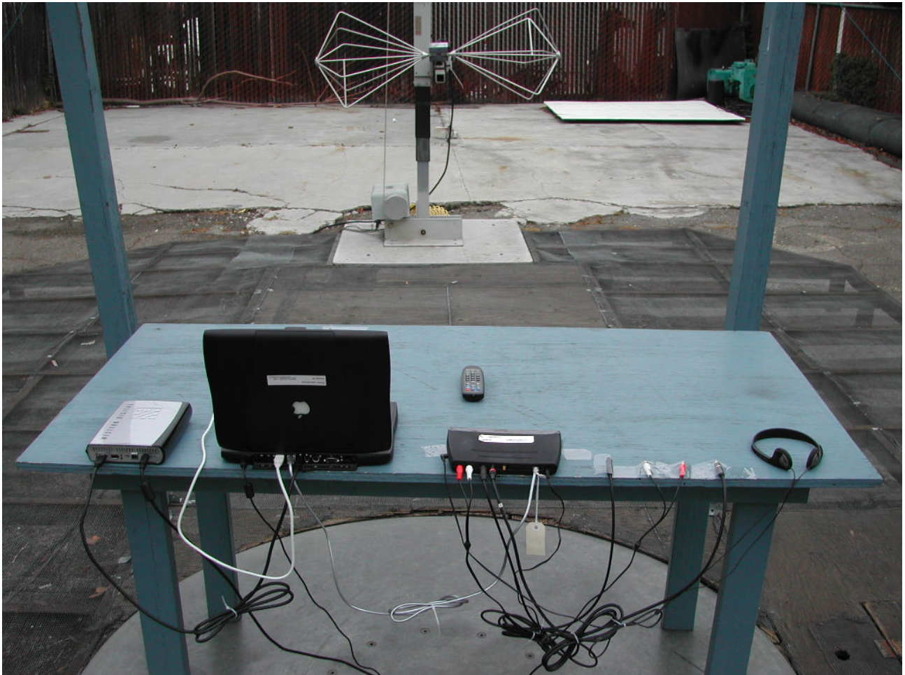
FIGURE 1: PLI Photograph Number 5392C3333SJ-02 illustrates the rear view of the Equipment Under Test in Radiated Electromagnetic Interference Test Configuration #1.
