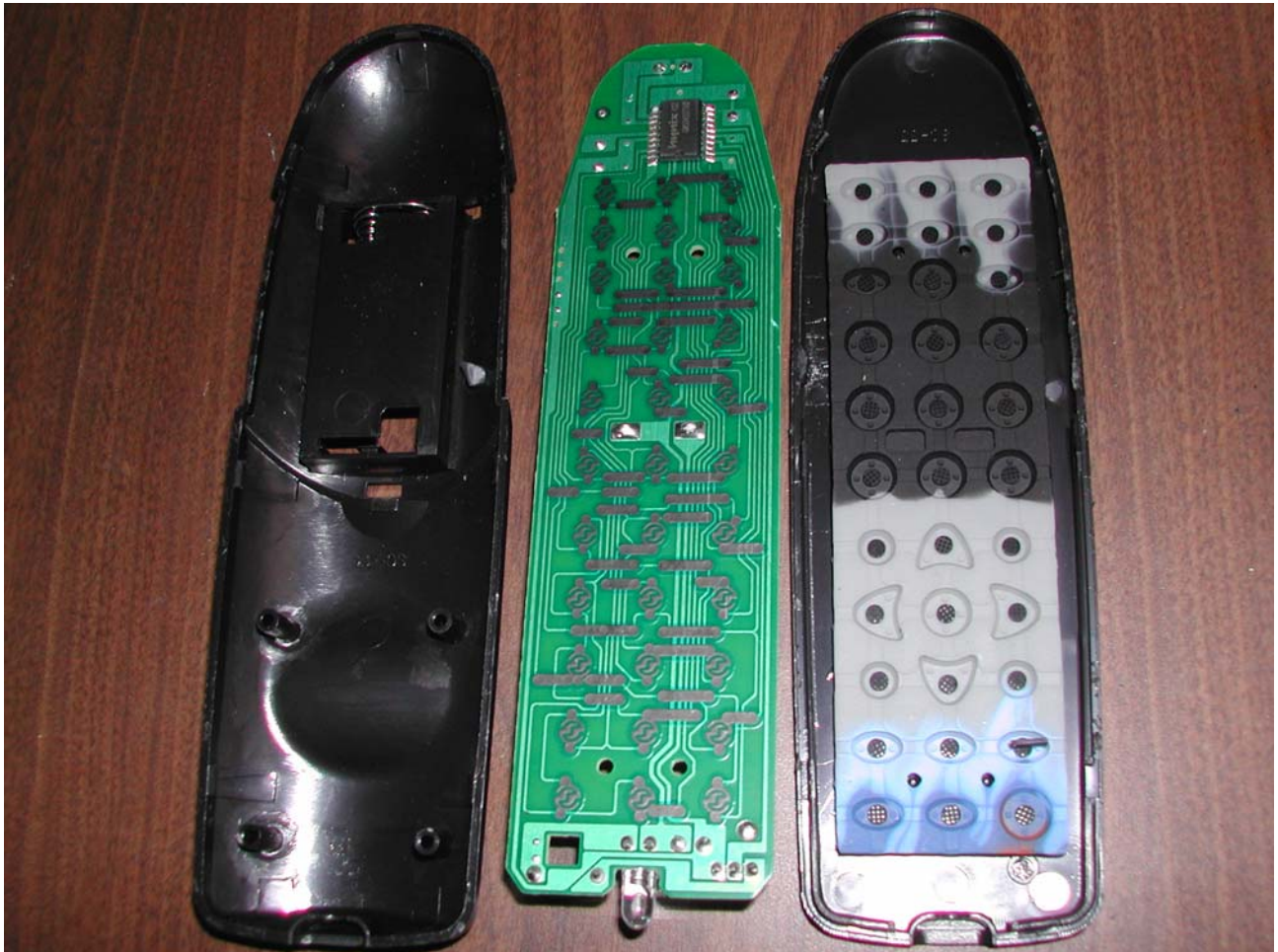
FIGURE 7: PLI Photograph Number 5392C2633SJ-15 illustrates the disassembled remote control and the circuit side of the remote control printed circuit assembly (assembly number S-251G203).
