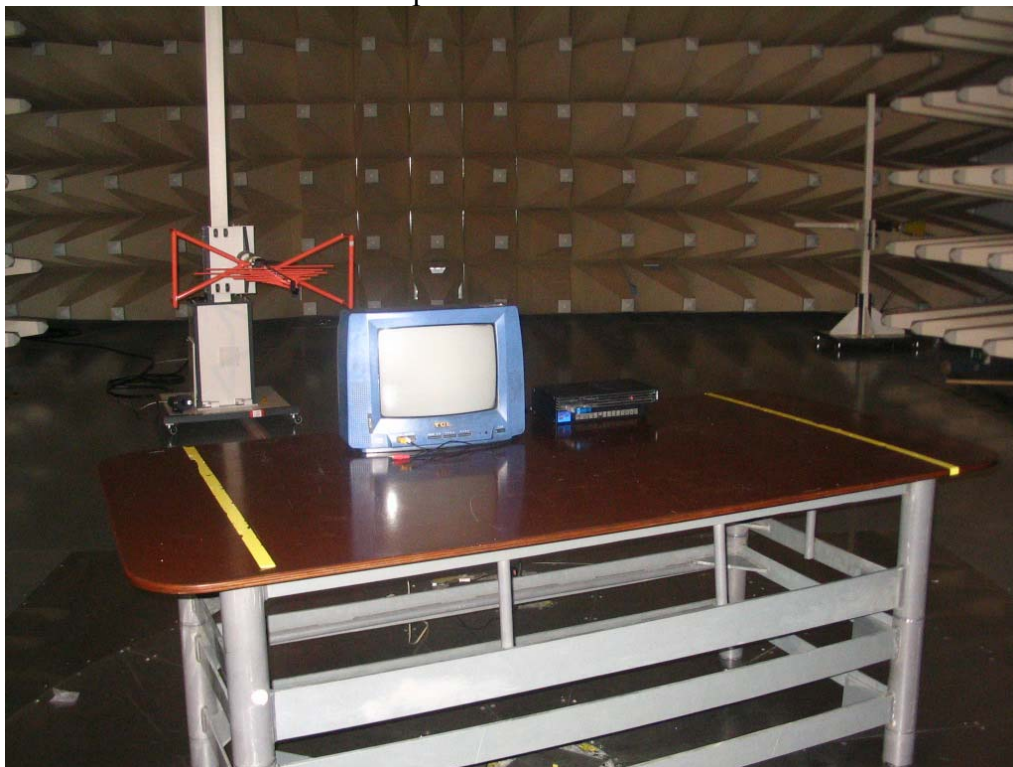
Radiated Emission Test Setup
