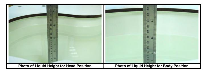
The dielectric properties of the head tissue simulating liquids are defined in IEEE 1528 and FCC OET 65 Supplement C Appendix C. For the body tissue simulating liquids, the dielectric properties are defined in FCC OET 65 Supplement C Appendix C. The dielectric properties of the tissue simulating liquids were verified prior to the SAR evaluation using an Agilent 85070D Dielectric Probe Kit and an Agilent Network Analyzer.
