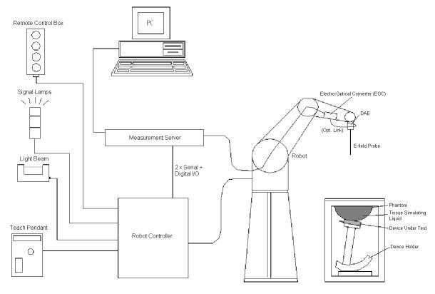
Fig-3.1 DASY System Setup
