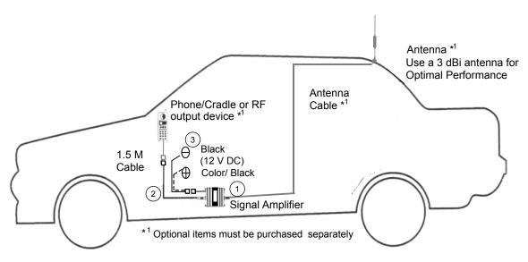
Typical Installation For Under The Seat Mounting
