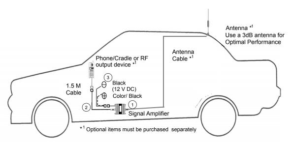
Typical Installation For Under The Seat Mounting
