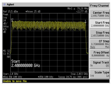
For GFSK mode Channel Spacing (Low CH=1MHz)
