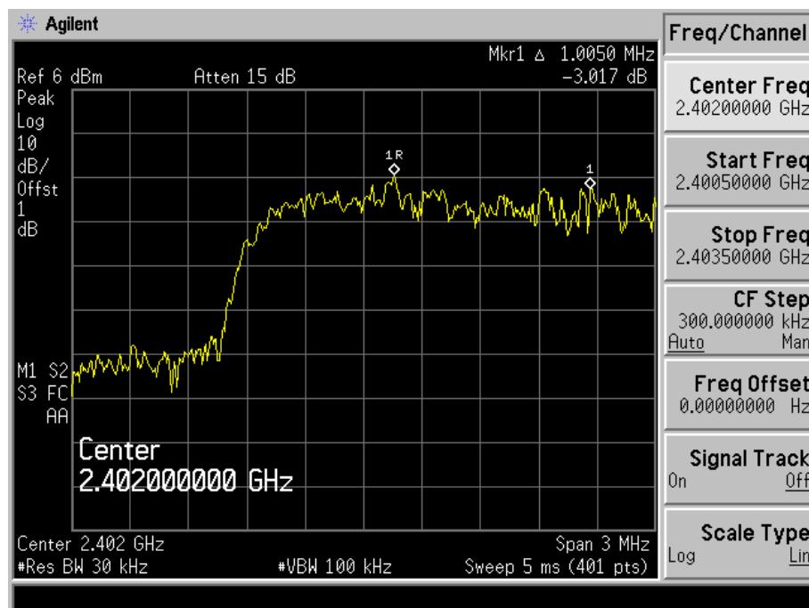
Channel Spacing (Middle CH=1MHz)
