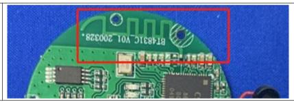
The antenna is PCB antenna. The best case gain of the antenna is 0 dBi.
