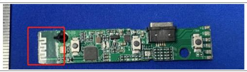
The antenna is PCB antenna. The best case gain of the antenna is 2 dBi.
