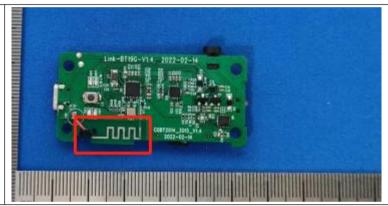
The antenna is PCB antenna. The best case gain of the antenna is 2 dBi.
