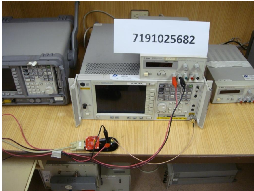
Carrier Frequency Separation Test Setup
