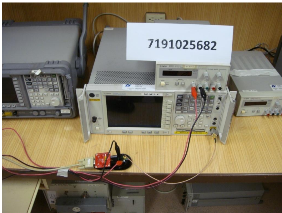
Average Frequency Dwell Time Test Setup
