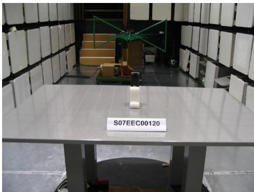
Radiated Emissions Test Setup (Rear View)
