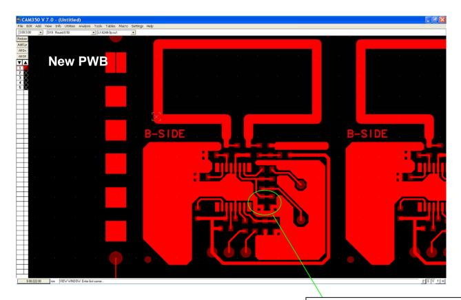
Two Pad added for two capacitor , to improve the Frequency stability
