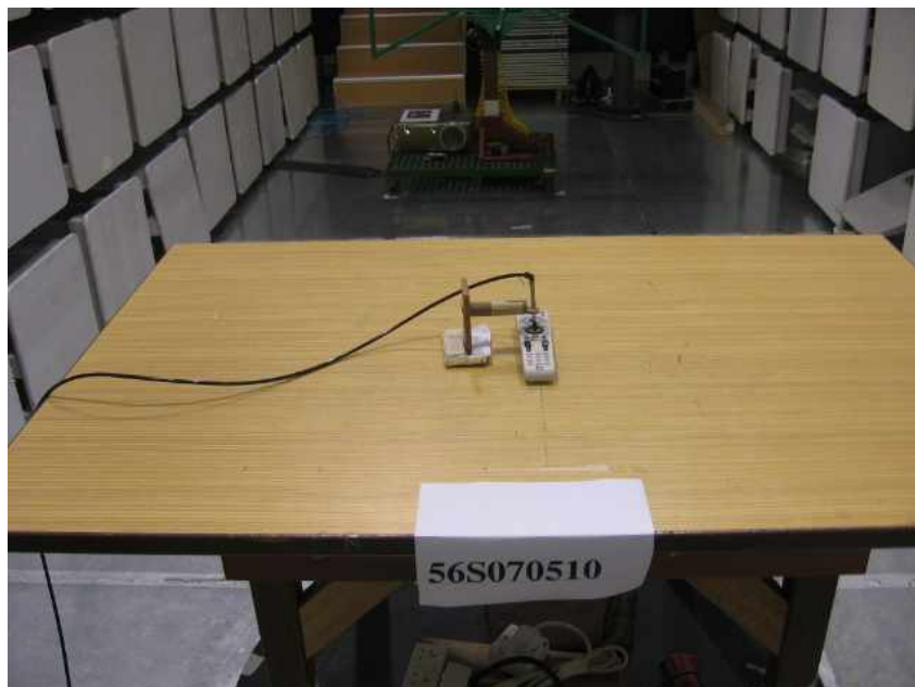
Radiated Emissions Test Setup (Rear View)
