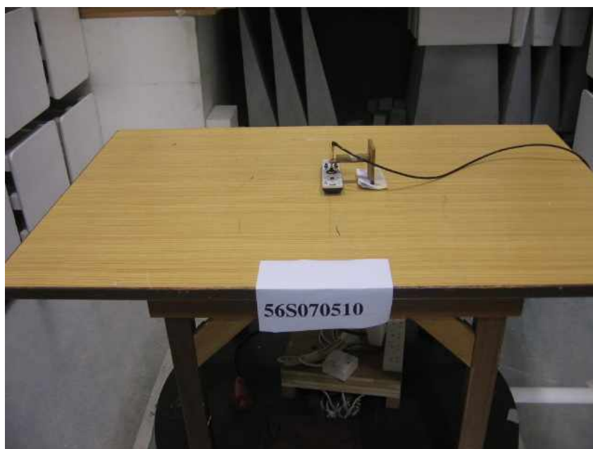
20dB Bandwidth Test Setup
