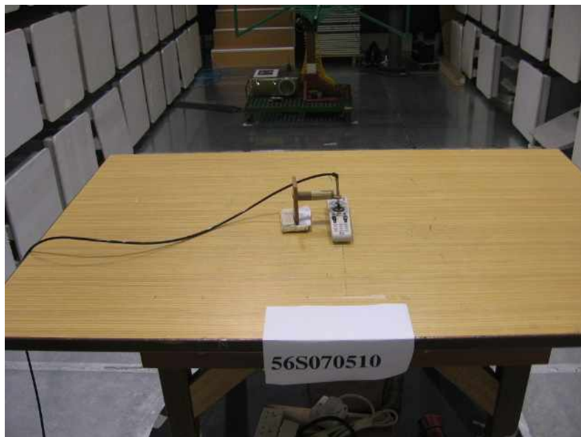
Radiated Emissions Test Setup (Rear View)
