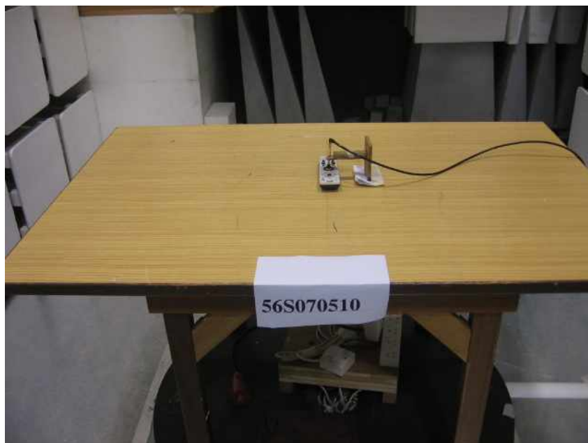
Radiated Emissions Test Setup (Front View)
