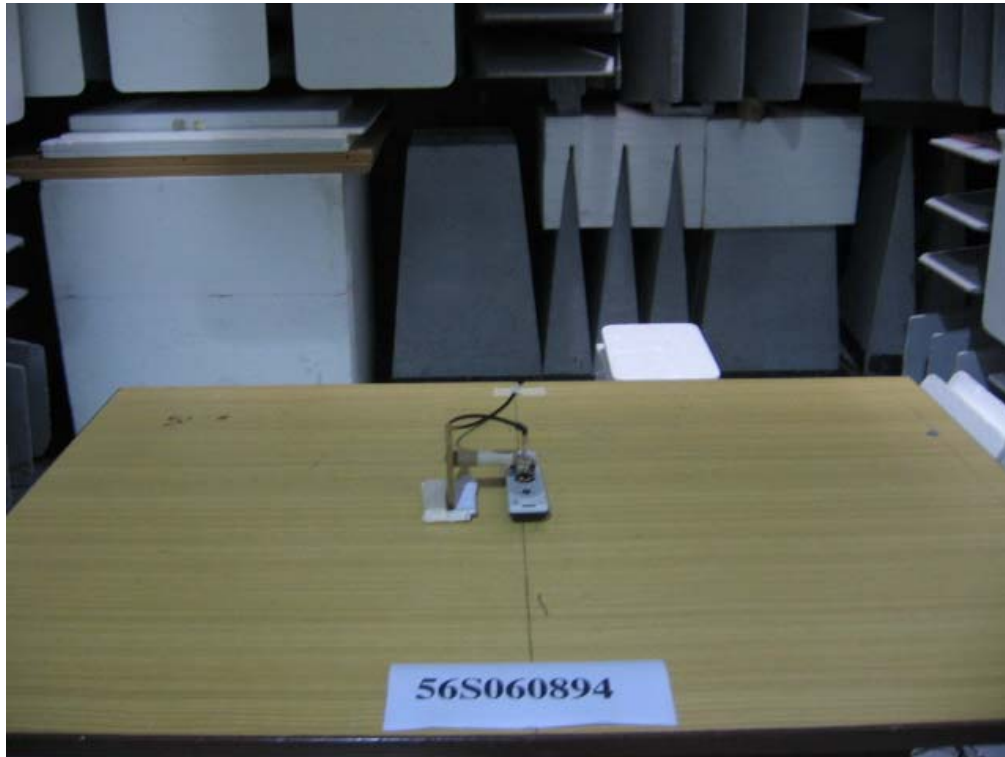
Radiated Emissions Test Setup (Front View)
