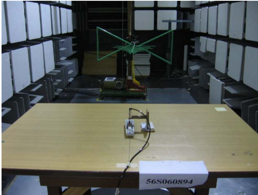
20dB Bandwidth Test Setup
