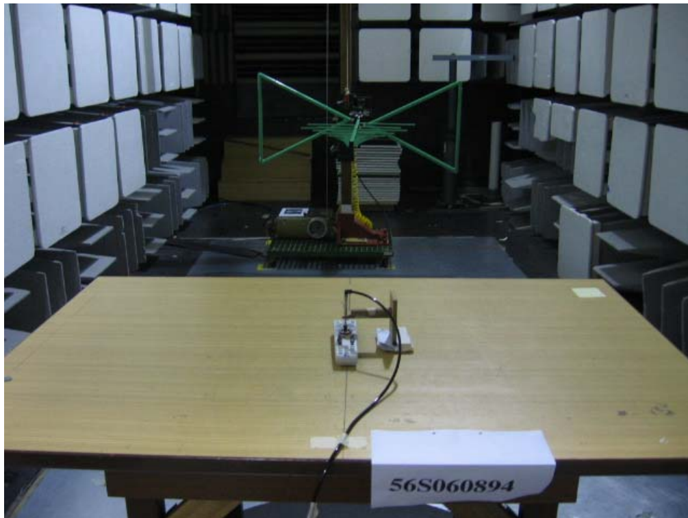
Radiated Emissions Test Setup (Rear View)
