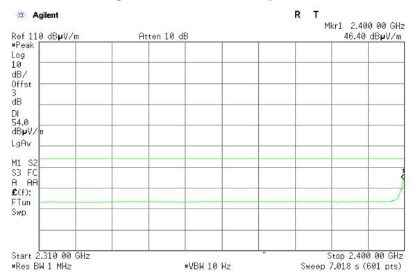
Detector mode: Peak Polarity: Horizontal
