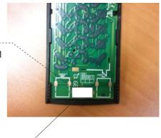
FACTORY PLATE to paste to the edge of PCB
