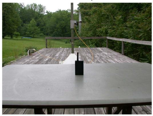
1 to 10 GHz Radiated Test Set-up for Transmitter
