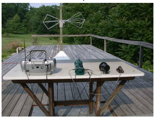
**Conducted Test Set-up for Receiver**
