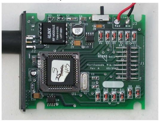
**Transmitter, Circuit Side of Printed Circuits Board**
