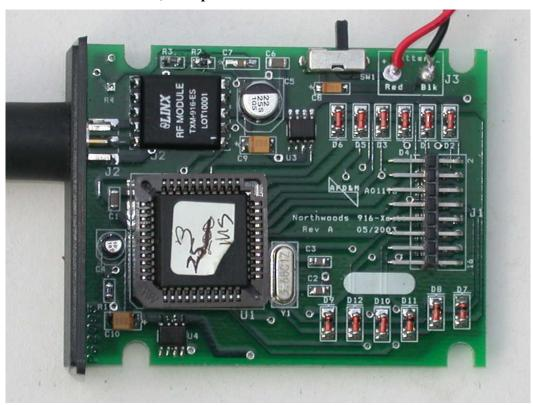
Transmitter, Circuit Side of Printed Circuits Board
