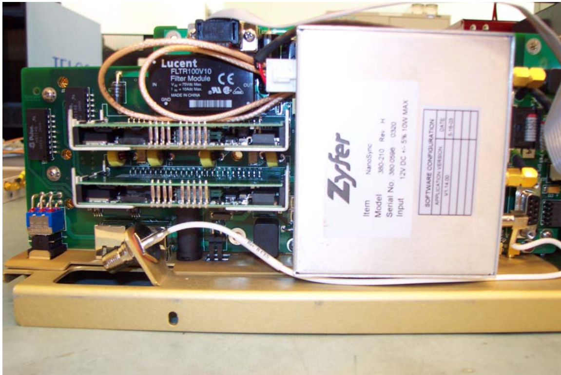
Front Power Supply Board
