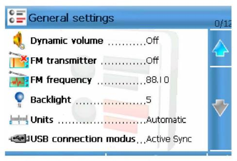
Go to Settings/General from main menu, there are two options for FM transmitter. Just tap the "FM transmitter" option to make sure the FM transmitter is turned on. You can also tap "FM frequency" option to set the frequency you want.
