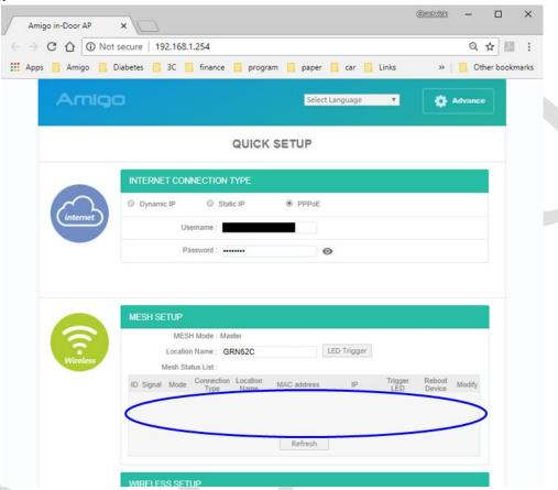
Solution: To push WPS buttons of fail Satellite and Master at the same time. Then they will be forced synchronization.
