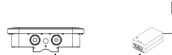
Note: The Access Point supports both IEEE 802.3at PoE (Power over Ethernet) or the included power adapter. You may use either one as the power source. DO NOT use both at the same time.
