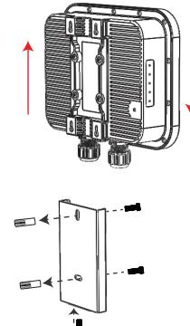
(2)Screw the anchors into the holes until they are flush with the wall.
