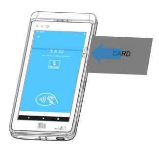
Bidirectional MSR capable of reading up to three tracks of data on ISO 7810/7811.
