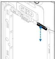
• Place the Micro SD and/or the Nano Sim card into the carrier with contact side face down.
