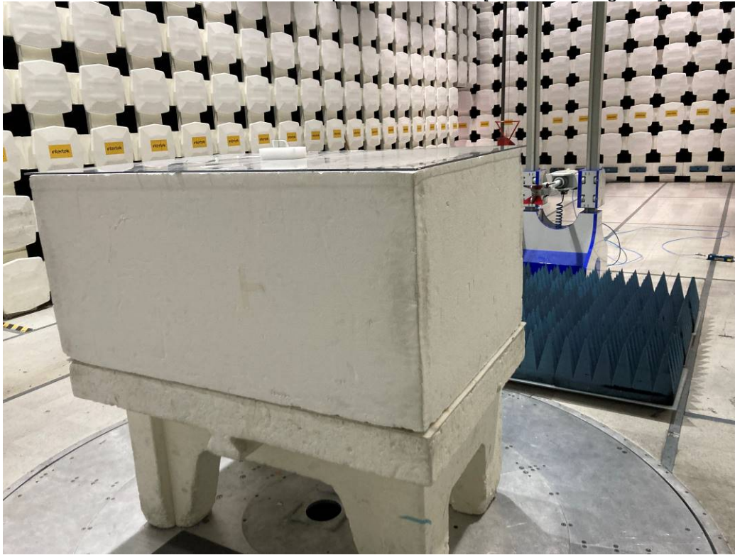
Radiated Emissions Test Setup From 1-18 GHz [EUT on its long side]
