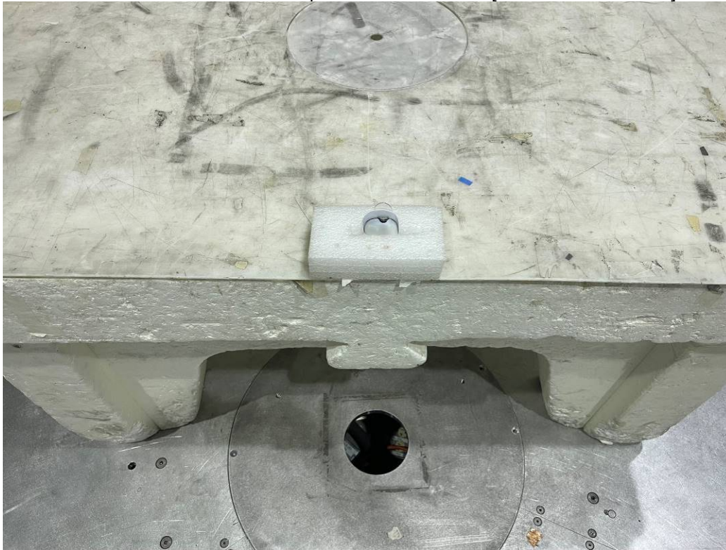
Radiated Emissions Test Setup From 30-1000 MHz [EUT on its short side]
