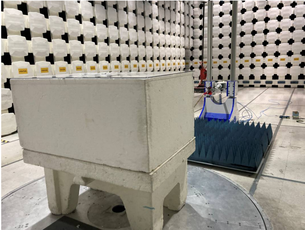
Radiated Emissions Test Setup From 1-18 GHz [EUT on its back]
