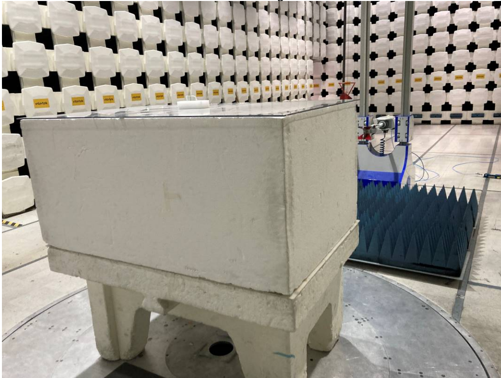
EUT on its long side
