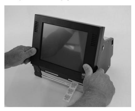
3. Rotate the display until it in a horizontal orientation as shown in the figure.
