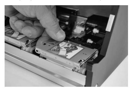
4. Rotate the printer mechanism cover to the open position as shown
