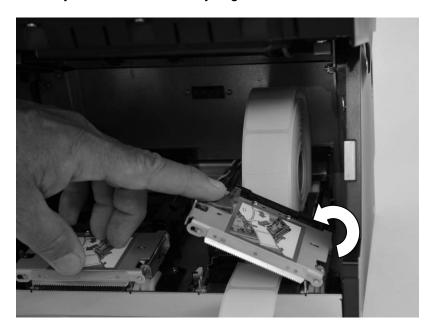
7. Grasp sides of display and rotate forward until it is in closed, latched position.
