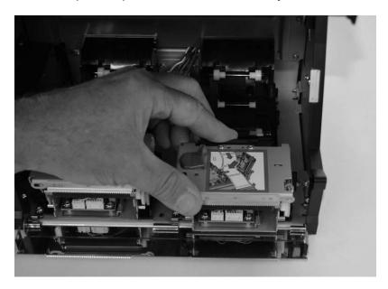
8. The printer mechanism is now removed.
