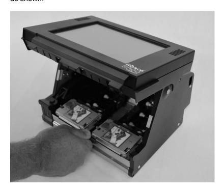
5. Rotate the door to the open position as shown in the figure.
