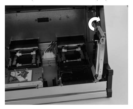
5. Drop the label roll into the label roll bucket. Note the proper orientation of label stock coming off **top** of roll.
