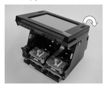
3. Grasp the plastic cover latch as shown and squeeze to release it.
