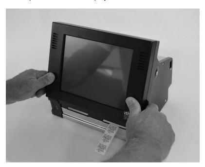
2. Rotate the display until it in a horizontal orientation as shown in the figure.
