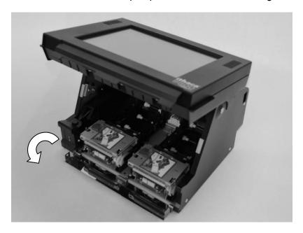
6. Lift and pull the printer mechanism carefully out of the terminal.
