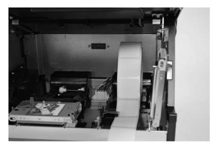
6. Close printer mechanism cover as shown. Rotate cover until it latches securely. Printer automatically aligns to the next label.
