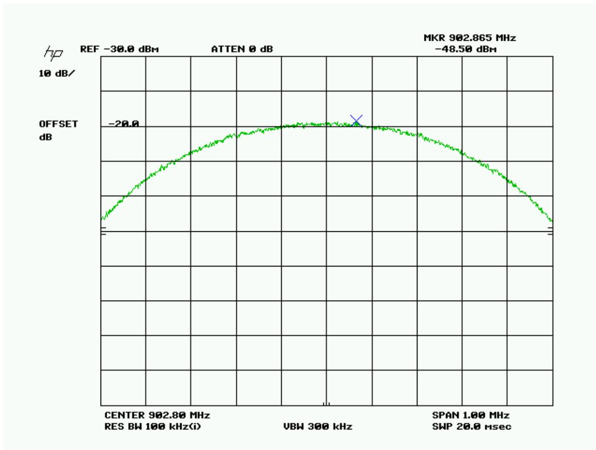
$$-11.0 \text{ dBm} + 20 \text{ dB (attn)} - 15.2 \text{ dB} = \text{PSD} -6.2 \text{ dB}$$
