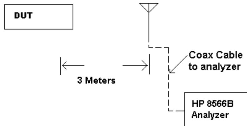
**METHOD OF MEASUREMENT:** The procedure used was ANSI standard C63.4-2003 & the FCC/OET Guidance on Measurements for Spread Spectrum Systems – KDB 558074 dated April 9, 2013.
