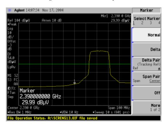
Detector mode: Peak Polarity: Horizontal
